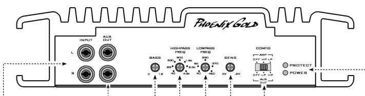
**AUXILIARY OUTPUTS** Provides either a low pass, high pass or full range signal for an additional amplifier or signal processor. The CONFIG SWITCH determines the state of the signal.
