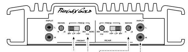
CROSSOVER CONFIG SWITCH This switch controls the type of signal that reaches the speaker ouputs. For a High Pass signal set the switch to HP. For Low Pass signal set the switch to LP. For a Full Range signal set the switch to BY.
