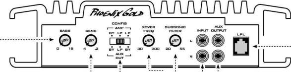
**INPUT SENSITIVITY** Used to reach maximum amplifier power with a wide variety of headunits. The amplifier is more sensitive to input signals when set to .2 and less sensitive when set to 4.
