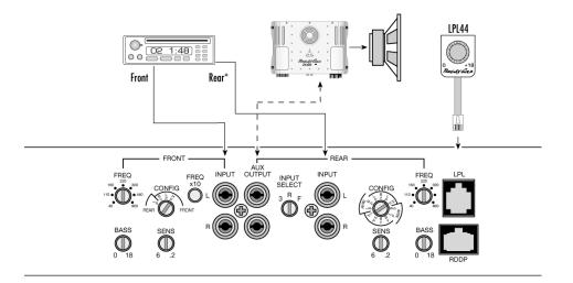
The front crossover frequency control determines the XS62's highpass frequency independently of the XS69's and auxiliary outputs.
