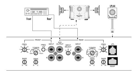
The front crossover frequency control determines the XS62's highpass frequency independently of the XS124 and rear speakers.
