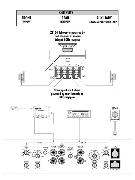
The auxiliary outputs send lowpass signals out to the Bass Cube and then back into the front inputs.
