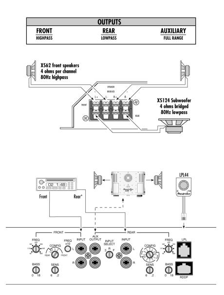
The front crossover frequency control determines the XS62's highpass frequency independently of the XS124 and rear speakers.
