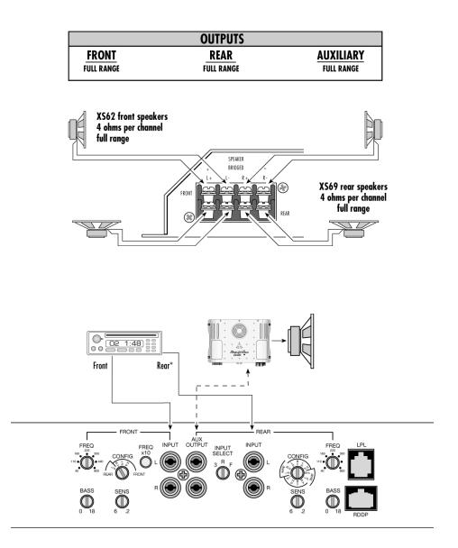
\* For single pre-amp headunits, set the input select switch to FRONT. This allows signal from the front inputs to reach the rear channels without the use of "Y" connectors.
