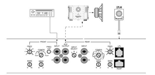
The front crossover frequency control determines the XS130's highpass.
