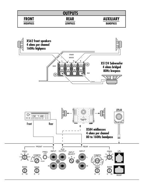
The front crossover frequency control determines the XS62's highpass frequency.
