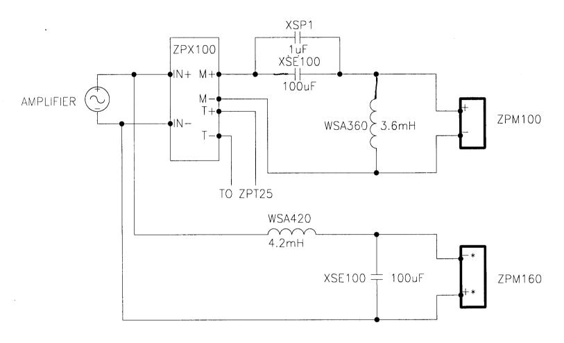
\* Experiment w/phase on ZPM160 for proper response.
