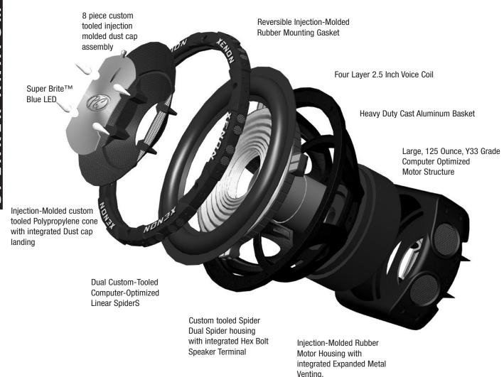
The **Xenon** subwoofer was developed from the ground up to compliment the amazing performance of our **Xenon** Series amplifiers. Utilizing cutting edge design techniques, we can deliver a woofer that has an impressive peak to peak linear field excursion of up to 40mm. The injection-molded 8 piece dust cap in conjunction with the custom injection-molded polypropylene cone provides
