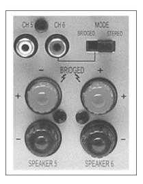
If you will be using the amplifier as a 12-channel (i.e.- not a bridged amplifier) you will connect the speakers positive (red) terminal to the amplifiers positive (red) terminal using the appropriate gauge speaker wire, and the speakers negative (black) terminal to the amplifiers negative (black) terminal (immediately below the positive terminal) using the appropriate gauge speaker wire. If you
