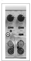
watts into 8 ohms. Any two adjacent channels may be bridged to provide a single more powerful channel rated at 180 watts into 8 ohm loads.
