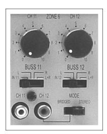
black knobs which correspond to the volume level of the channel identified by a channel number above it. The volume range is labeled 0-10 and has 40 steps (clicks) from minimum to maximum output. Rotate the knob clockwise to increase output, and counterclockwise to decrease output.
