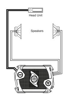
Figure 5: Bridged Single Woofer Connection
