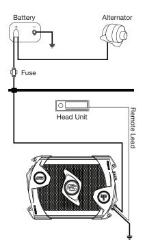
Figure 4: Stereo Connection
