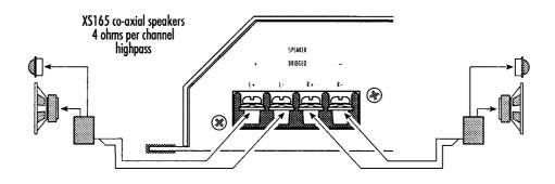
Minimum bridged load is 2 ohms. Minimum load per channel is 1 ohm.
