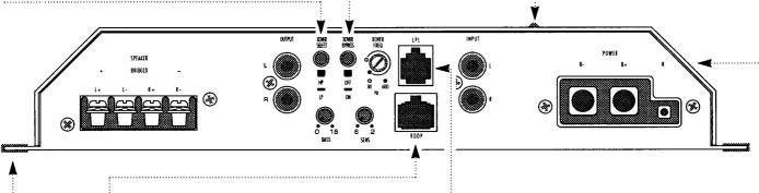
**REMOTE DIAGNOSTIC DISPLAY PORT** This port is for connecting the optional Remote Diagnostic Display. The display indicates the amplifier's condition with additional status LEDs and a DC voltmeter.
