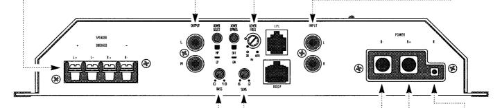
BASS EQ This control allows up to 18dB of boost at 45Hz for the speaker outputs. It cannot affect the auxiliary outputs. Use this control sparingly. Every 3dB of boost requires double the power at 45Hz.
