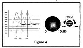
down, "counter -clock-wise"(see Figure 4). Remember that this "FREQ" knob works through a range of 20 to 110Hz. As you adjust the "FREQ" knob you will notice the bass level changing. With a vented
