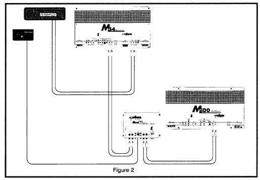
need subwoofers, although it makes for more impressive results if they are there. For this conversation we'll place the BassCube after the subwoofer line out of the 4-channel amplifier, before the sub amplifier (see Figure 2). After mounting the BassCube near the amplifier and doing the normal cable
