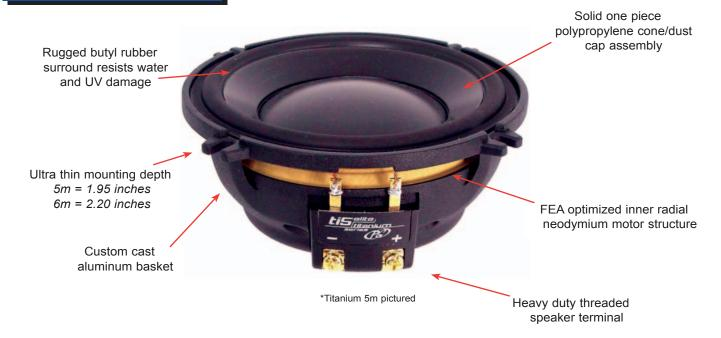
The Titanium Elite series midranges are design to give the ultimate acoustic performance in a small efficient space. By utilizing an inner radial motor structure we can "hide" all of the magnetic material inside of the voice coil which provides for a shallow mounting depth and greatly improved acoustical performance. The motor is designed around a 3" neodymium slug that sits inside of the
